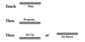
After either pad is touched once, time will advance or decrease in one minute increments. Press either pad again to stop the display's time setting cycle.
