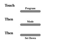
When the control panel lock is engaged, all automatic spa functions will operate normally but cannot be altered. To unlock the panel, the three pads must be pressed in the correct sequence and within **three seconds**. When the last pad is pressed, the lock symbol will disappear. All pads are now active.
