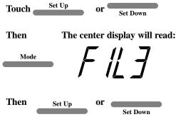
Adjust the cycle duration by pushing the set up or set down pad. Each press of the pad will display which filtration cycle you have chosen:
