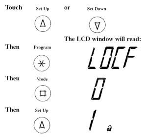
To activate the Temperature Lock feature, this sequence must be done within three seconds. The LCD window will display the water temperature along with the lock symbol. Both temperature pads will be deactivated and when pushed, the set temperature will appear in the LCD window next to a double arrow.
