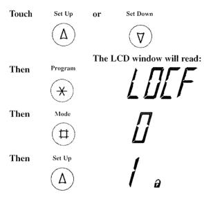
To activate the Temperature Lock feature, this sequence must be done within three seconds. The LCD window will display the water temperature along with the lock symbol. Both temperature pads will be deactivated and when pushed, the set temperature will appear in the LCD window next to a double arrow.
